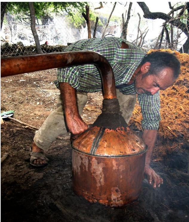
Aquilino has a copper still that has a 250-liter capacity. He makes all the separations (cuts) by smell and taste. The heads are between 70% and 30% AVB and his tails are between 30% and 15% AVB. Everything else he doesn't use.
